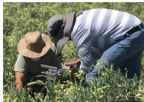
Soil moisture probe installation
