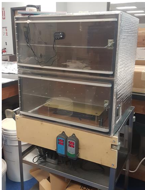
Photo 10. Environmental control chamber built for experiments in Tucson, Arizona.
