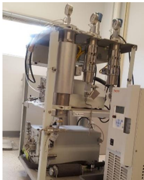
Photo 8. Supercritical fluid extraction system in high-pressure equipment lab, awaiting installation of blast shields, workstation, and cryogen tanks.
