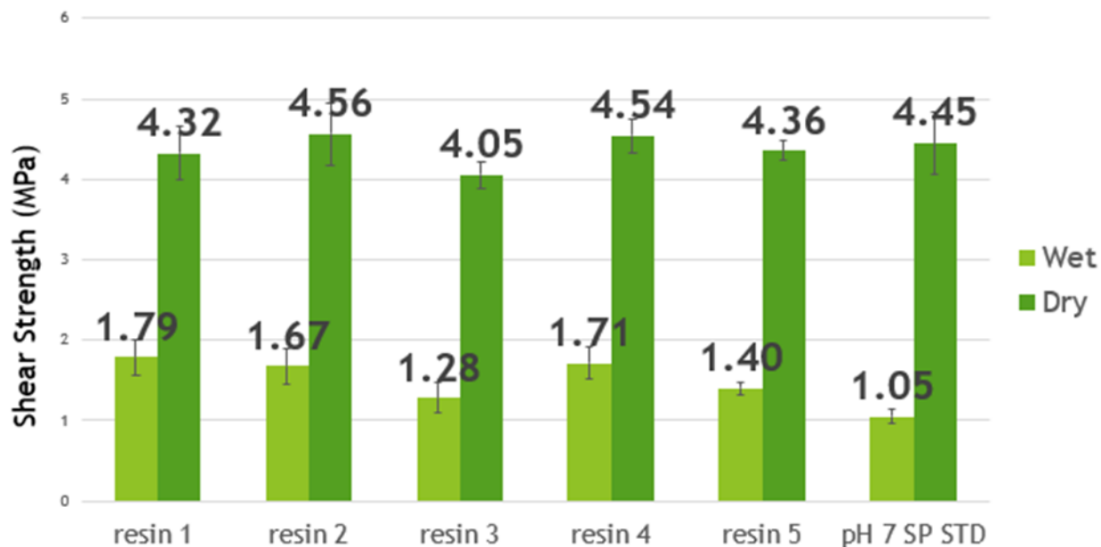
Figure 12. Wet and Dry adhesion strength of soy protein adhesive used with Resin samples: 1, 2, 3, 4, and 5.
